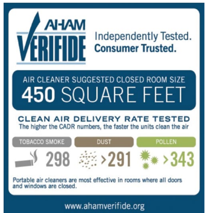
Figure 5. Example of a label from a portable air cleaner. 5 Note: this label uses square feet, assuming an 8 foot ceiling. In rooms with ceiling greater than 8 feet, the calculation needs to be adjusted downward or multiple air cleaners should be used.
